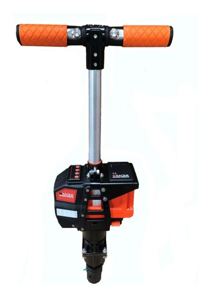
The Battery I" T-Handle Impact Wrench is a portable, 36VDC Lithium Ion battery powered, quality tool with unique features that make it the perfect solution for installing and removing lag screws and Vohsloh® style rail clips.
